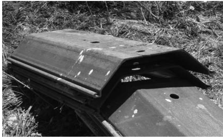
Figure 4.4 Some steel sheet piles at a construction site (Courtesy of N. Sivakugan, James Cook University, Australia)
